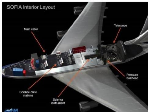
Built within the frame of a Boeing 747SP, SOFIA contains an internally mounted 2.7-meter (approximately 9-foot) telescope that operators expose to the night sky through a uniquely designed cavity door located at the rear of the plane. NASA designed SOFIA to observe both infrared and visible wavelengths from 0.3 to 1.600 microns.
